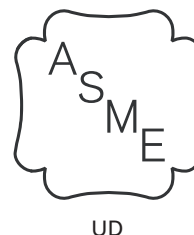
Figure UG-129.2 Official Certification Mark to Denote the American Society of Mechanical Engineers' Standard for Nonreclosing Pressure Relief Devices
